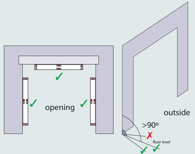
The threshold must be flat/level and sound across the full width of the opening.
